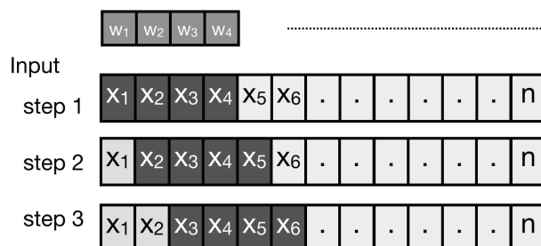
Figure 13. An example of a convolutional filter that convolves over the input. Its window size is four and it strides by one at each step.
