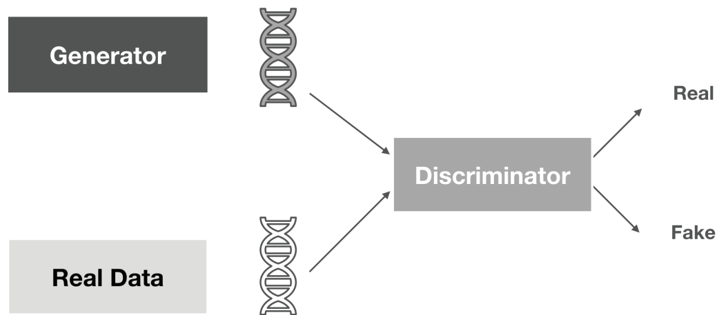
Figure 17. An illustrative example of how the GAN architecture is trained. The Generator tries to synthesize sequences, while the Discriminator tries to distinguish between the real and fake ones.
