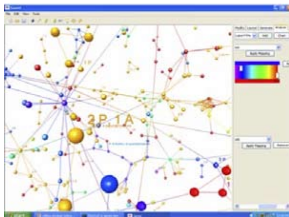
Figure 1. Screenshot of GEOMI, a network visualisation tool developed by Dr. Seokhee Hong (National ICT Australia). This version of GEOMI has been specifically tailored by the SBI to allow co-visualisation of protein- protein interaction networks or complexome networks with multiple protein parameters (e.g. abundance, half-life, function, localization) or gene expression data.
