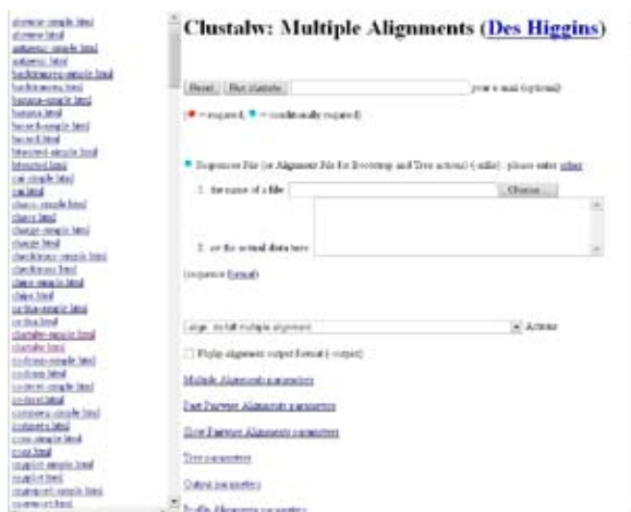
Figure 7. An example of the PISE web interface generated on our cluster. PISE automatically queues the processes on SGE in a transparent way for users.
